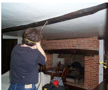
Photo 5: Extraction of a core in progress
